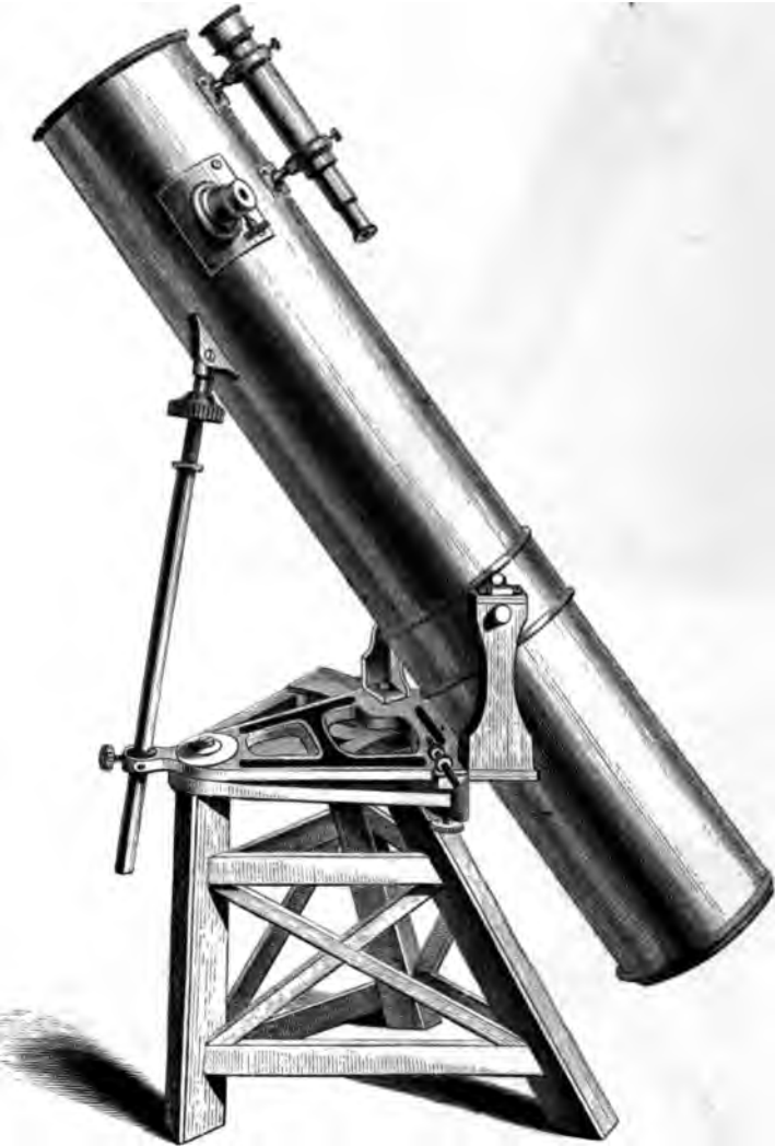
ALTAZIMUTH MOUNTING FOR A LARGE REFLECTOR. ( By Browning. )
